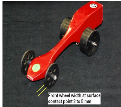
(S) Wheels: Front width at surface contact point
